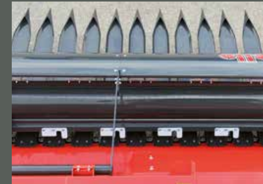
The spoon-shaped divider points are made from wear-resistant steel.
