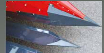
The spoon-shaped divider points are made from wear-resistant steel.
